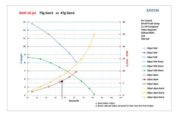
Step 4 – From the "grams/hr" scale move vertically to The "10 psi slpm" graph line.
