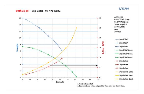
Step 5 – From the "10psi slpm" graph line, move horizontally to the "O2 Flow SLPM" scale. This indicates An oxygen flow of just over 5 SLPM. *In summary this graph example indicates 10% weight ozone at 47 g/hr takes just over 5 SLPM of oxygen.*
