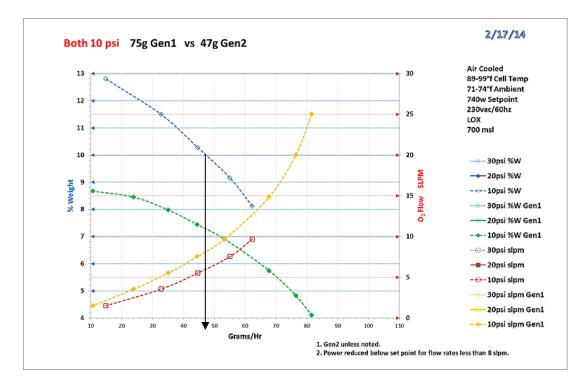
Step 3 – Move down to the "grams/hr" scale. This example indicates 47g/hr at 10% weight.
